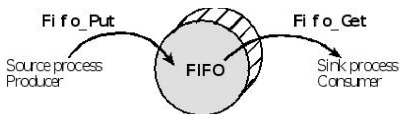
Figure 3.9. The FIFO is used to buffer data between the producer and consumer.
