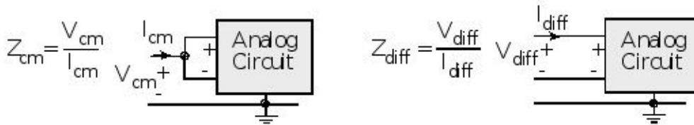
Figure 8.9. Definition of input impedance for an analog circuit with two inputs.
