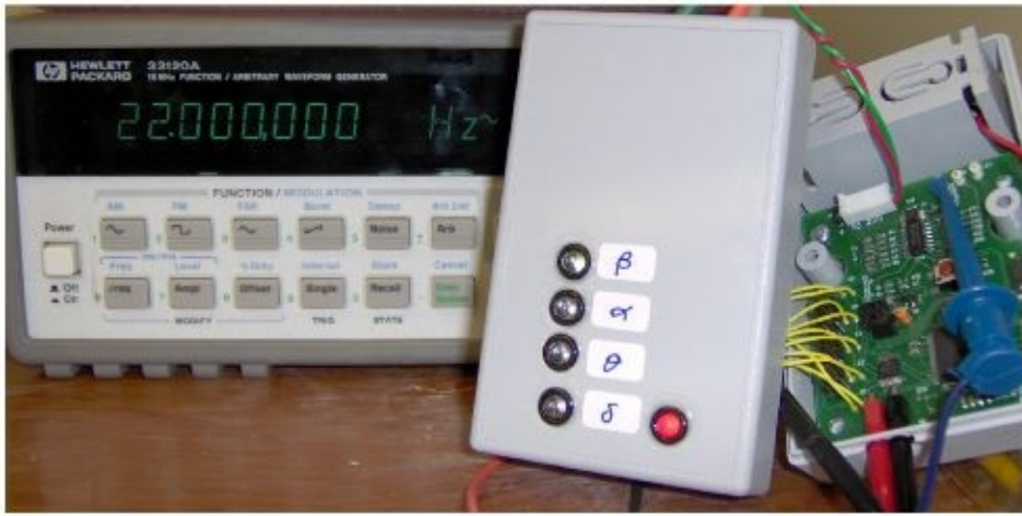
Figure 9.8. An EEG system designed with a LM3S8962 that fits into a case (designed by Katy Loeffler).
