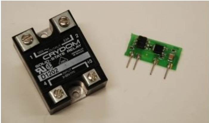
Figure 6.18. Solid state relays can be used to control power to an AC appliance.
