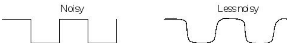
Figure 10.24. Limiting rise/fall times can reduce radiated noise.
