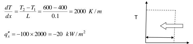
**Example2**: Find  $\frac{dT}{dx}$  and thermal conductivity of the following figure?
