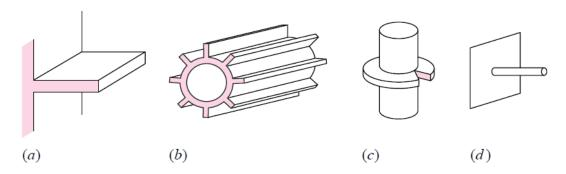
For rectangular fin having a temperature  $T^{\circ}$  at the base surrounded by a fluid temperature  $T^{\infty}$ Energy in left face = energy out right face + energy lost by convection.
