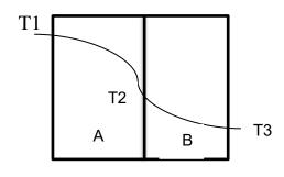
$$Heat flow = \frac{thermal potential difference}{thermal resistance}$$
