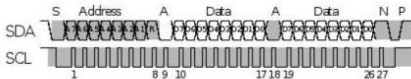
Figure 5.10. I2C transmission of two bytes from slave to master.
