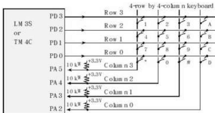
Fig. 5.6 A matrix keyboard interfaced to the microcomputer.
