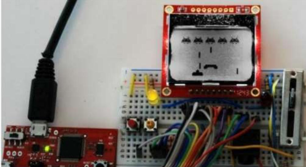
Fig. 5.4 Nokia 5110 display with 84 by 48 monochrome pixels.
