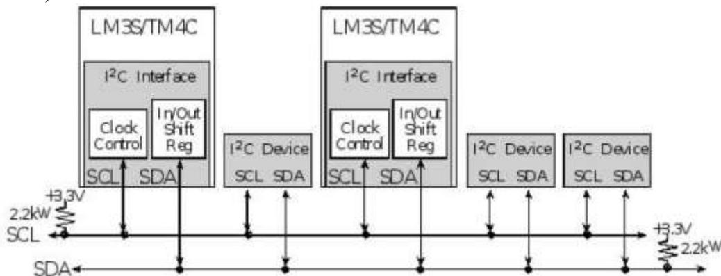
Figure 5.7. Block diagram of an I2C communication network.
