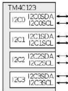
Figure 5.12. I/O port pins for I2C on various LM3S/TM4C microcontrollers.
