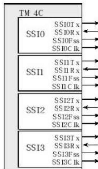
Fig. 5.1 Synchronous serial port pins on Stellaris ® TM4C microcontrollers.
