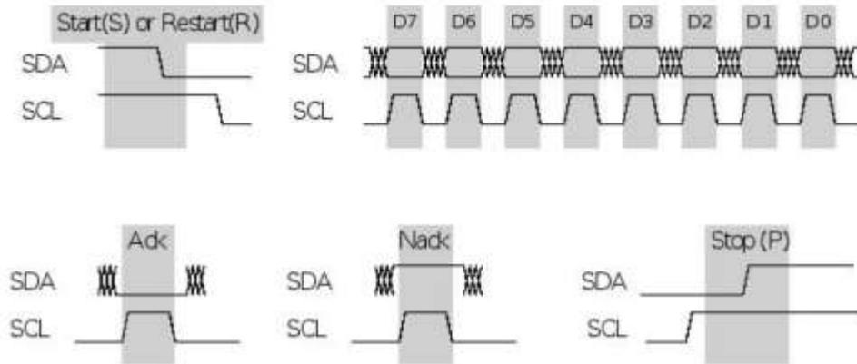
Figure 5.8. Timing diagrams of I2C components.
