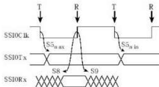
Figure 5.3. Synchronous serial timing showing the data available interval overlaps the data required interval.
