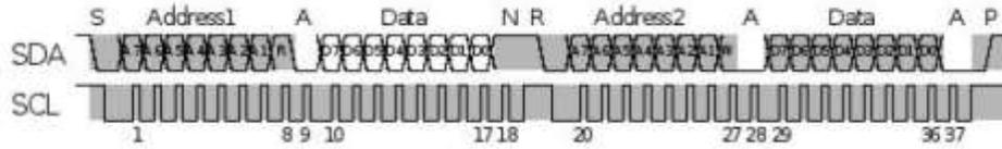
Figure 5.11. I2C transmission of one byte from the first slave and one byte to a second slave.
