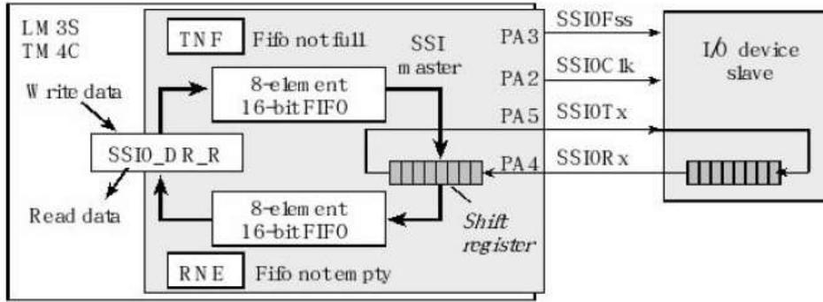
Figure 5.2. A synchronous serial interface between a microcontroller and an I/O device.
