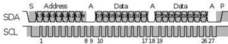
Figure 5.9. I2C transmission of two bytes from master to slave
