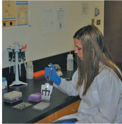
(a) A technician uses a micropipette to add samples to a microplate for an ELISA.
