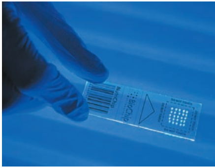
(a) A DNA chip can be manufactured to contain hundreds of thousands of synthetic single-stranded DNA sequences. Assume that each DNA sequence was unique to a different gene.
