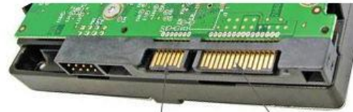
SATA Data Connector Hard Disk Power Connector
