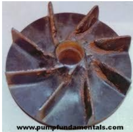
Fig.12 Cavities in pump impeller
