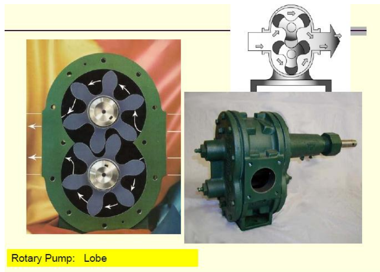
Fig.3 Rotary pump
