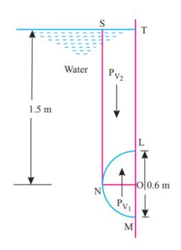
Vertical force,  $F_V = F_{V_1} - F_{V_2}$ = Weight volume of water MNST – weight of volume of water LNST = Weight of water contained by the hemisphere LNM =  $w \times \frac{1}{2} \left(\frac{4}{3} \pi R^3\right)$ =  $9.81 \times \frac{1}{2} \times \frac{4}{3} \times \pi \times (0.3)^3$ = 0.555 kN (Ans.) Horizontal force,  $P_H = wA\overline{x}$ =  $9.81 \times \pi \times (0.3)^2 \times 1.5 = 4.16 \text{ kN}$  (Ans.)
