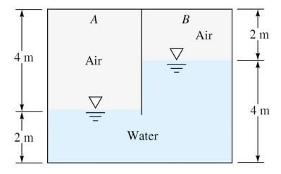
**Solution:** First compute  $\rho_A = p_A/RT = (95000)/[287(293)] \approx 1.13 \text{ kg/m}^3$ , hence  $\gamma_A \approx (1.13)(9.81) \approx 11.1 \text{ N/m}^3$ . Then proceed around hydrostatically from point A to point B:
