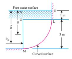
**Example:** Find the force F required to hold the gate in the position shown in figure. The gate is 5 m wide.
