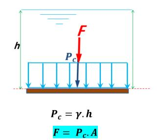
$y_p = h_{\blacksquare} = y_c$ where :  $P_c = pressure$  at the gate centroid =  $\gamma . h_p$  for same fluid
