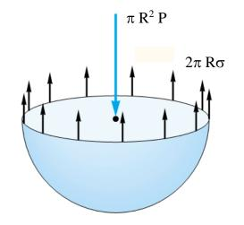
For a *Soap(or hollow)bubble*: Soap bubbles have two surfaces on which surface tension  $\sigma$  acts. free body gives:
