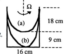
b) The bottom is barely exposed if the paraboloid surface is 27 cm deep:
