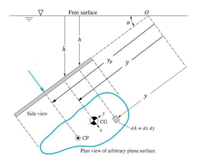
Cp: Center of pressure force CG: center of geometry The total force of the liquid on the plane surface is found by integrating the pressure over area.
