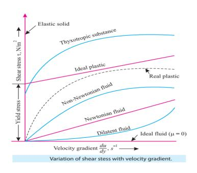
2. Non-Newtonian fluids: Fluids which *do not follow* the linear relationship between shear stress and rate of deformation. Such fluids are relatively uncommon. Examples. Solutions or suspensions (slurries), mud flows, polymer solutions, blood etc.
