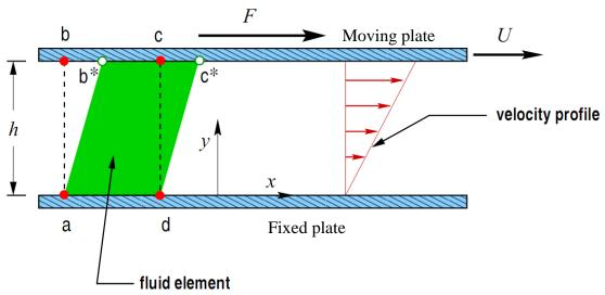
The fluid in the area a-b-c-d flows to the new position  $a-b^*-c^*-d$ , each fluid particle *varying uniformly from zero at the fixed plate to U* at the moving plate.
