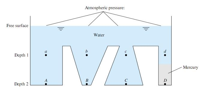
Points *a*, *b*, *c*, and *d* are at equal depths in water and therefore have identical pressures. Points *A*, *B*, and *C* are also at equal depths in water and have identical pressures higher than *a*, *b*, *c*, and *d*. Point **D** has a different pressure from *A*, *B*, and *C* because it is not connected to them by a water path.
