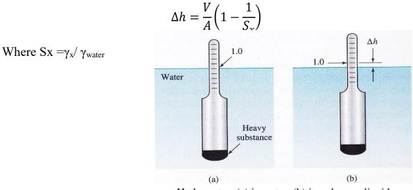
Hydrometer: (a) in water, (b) in unknown liquid
