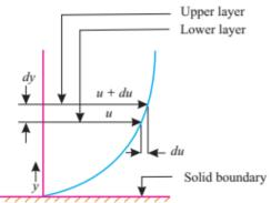
Now,  $\mu$  is called the viscosity (or dynamic viscosity) of fluid, and the relation above is the *Newton's law of viscosity*.
