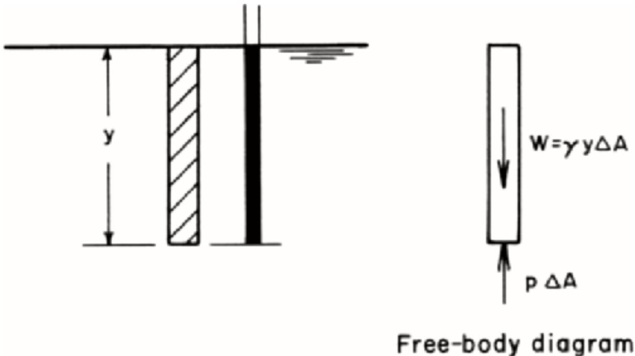
**Fig . 6 Pressure in stationary fluid**
