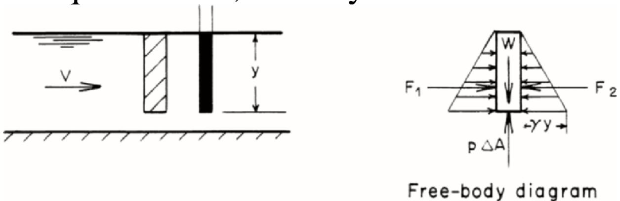
**Fig. 7 Horizontal, parallel flow**
