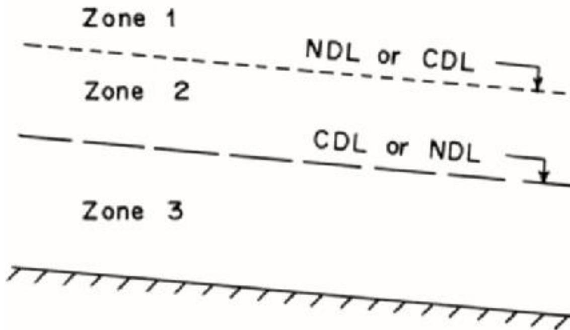
**Fig 3-2 Zones for classification of surface profiles**
