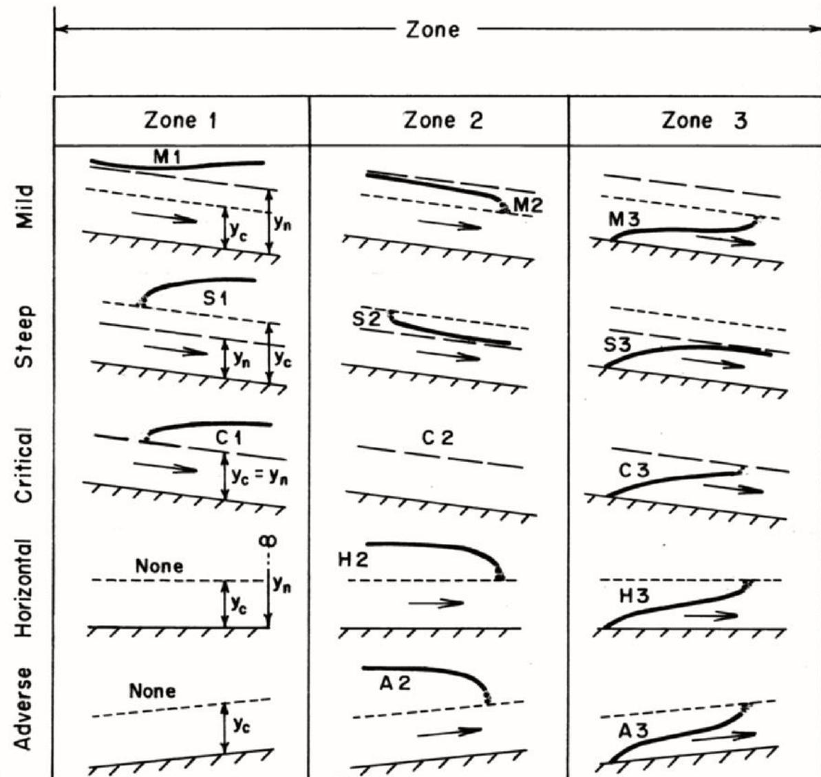
**Fig. 3-3 Water surface profiles**
