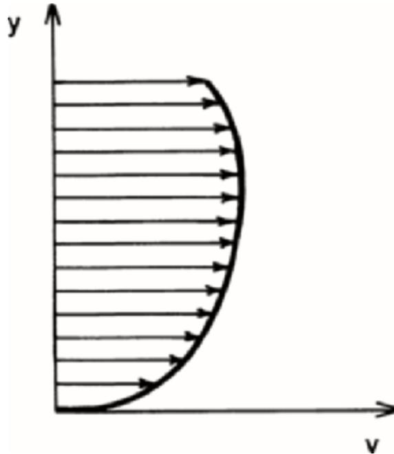
**Fig. 3 Typical velocity variation with depth**
