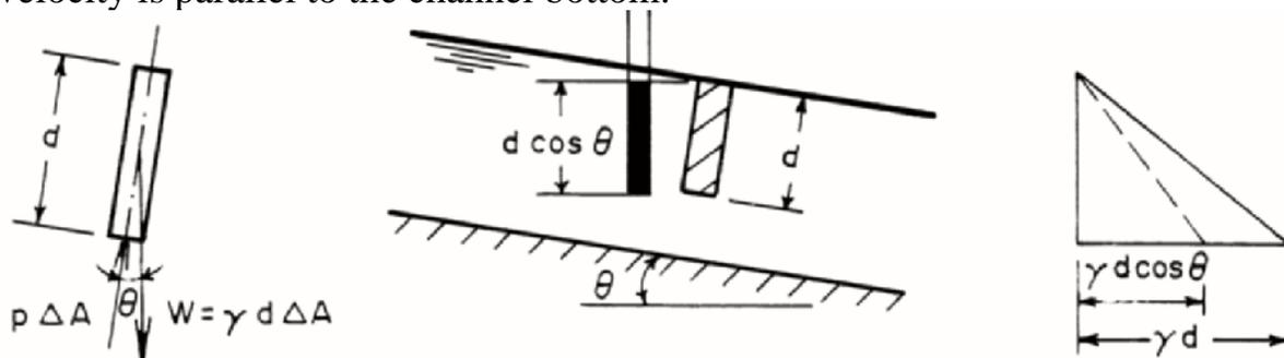
**Fig. 8 Parallel flow in a sloping channel**
