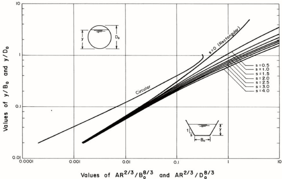
Fig 3 Curves for the computation of normal depth
