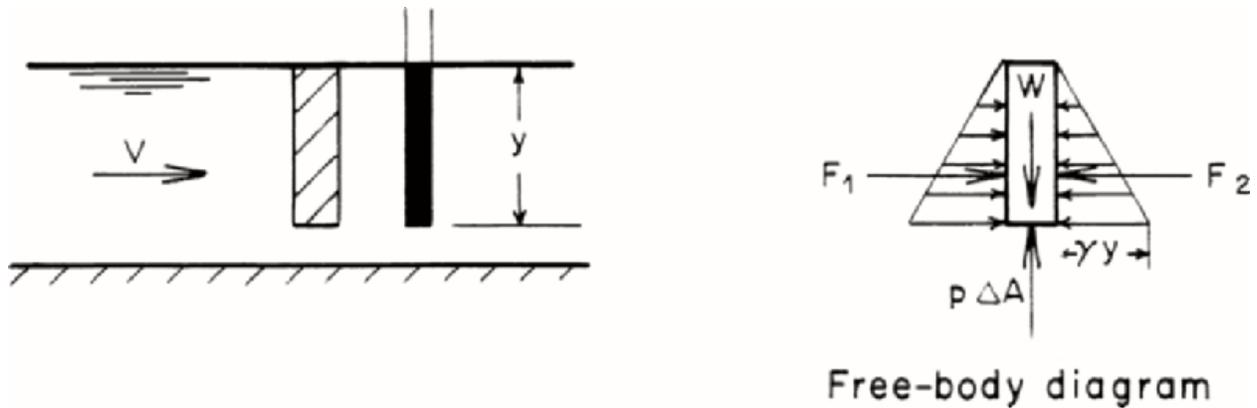
**Fig. 7 Horizontal, parallel flow**
