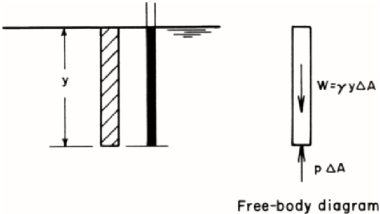
**Fig . 6 Pressure in stationary fluid**
