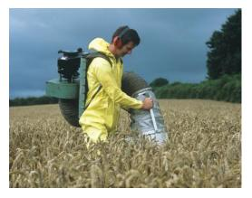
Figure 2.15 D-vac mechanical vacuum sampler used to collect small arthropods—in this instance, in a ripe wheat field.
