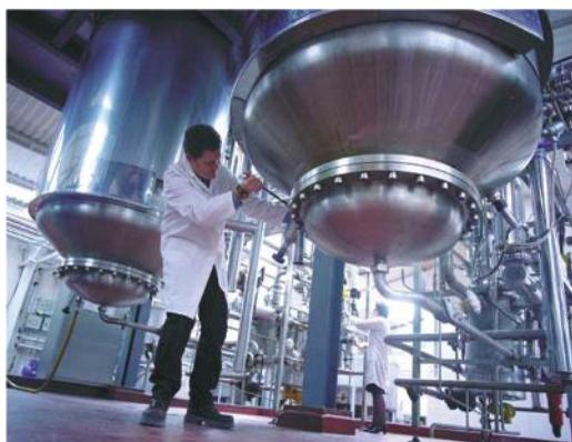
**Figure 1.6** Large-scale fermenters for nematode production. (Photograph courtesy of BASF Agricultural Specialties, Littlehampton, W. Sussex, UK.)
