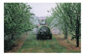
Figure 2.22 Tractor-driven, air-assisted sprayer treating an apple orchard, Provence, France.
