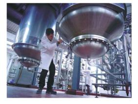
Figure 1.6 Large-scale fermenters for nematode production. (Photograph courtesy of BASF Agricultural Specialties, Littlehampton, W. Sussex, UK.)
