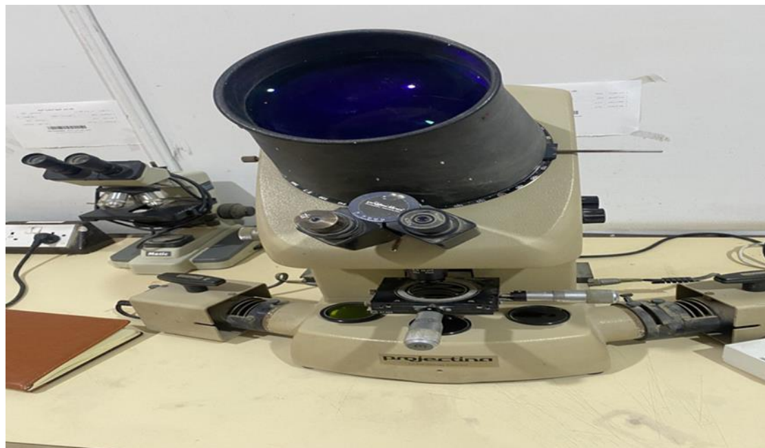
Plot. 1. Device Projectina to Examine and Enlarge Plastic Particles
