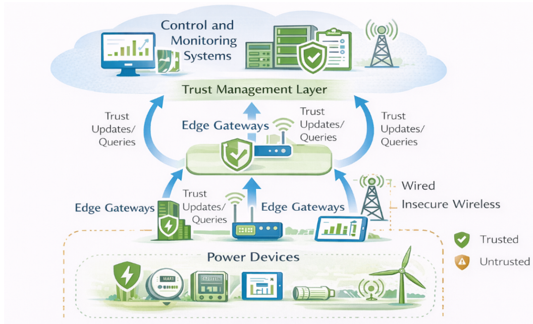
Fig. 1. System model for the proposed energy-efficient cryptographic trust framework in power systems
