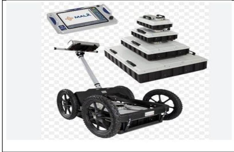
Plate 1. GPR main equipment MALA GX System
