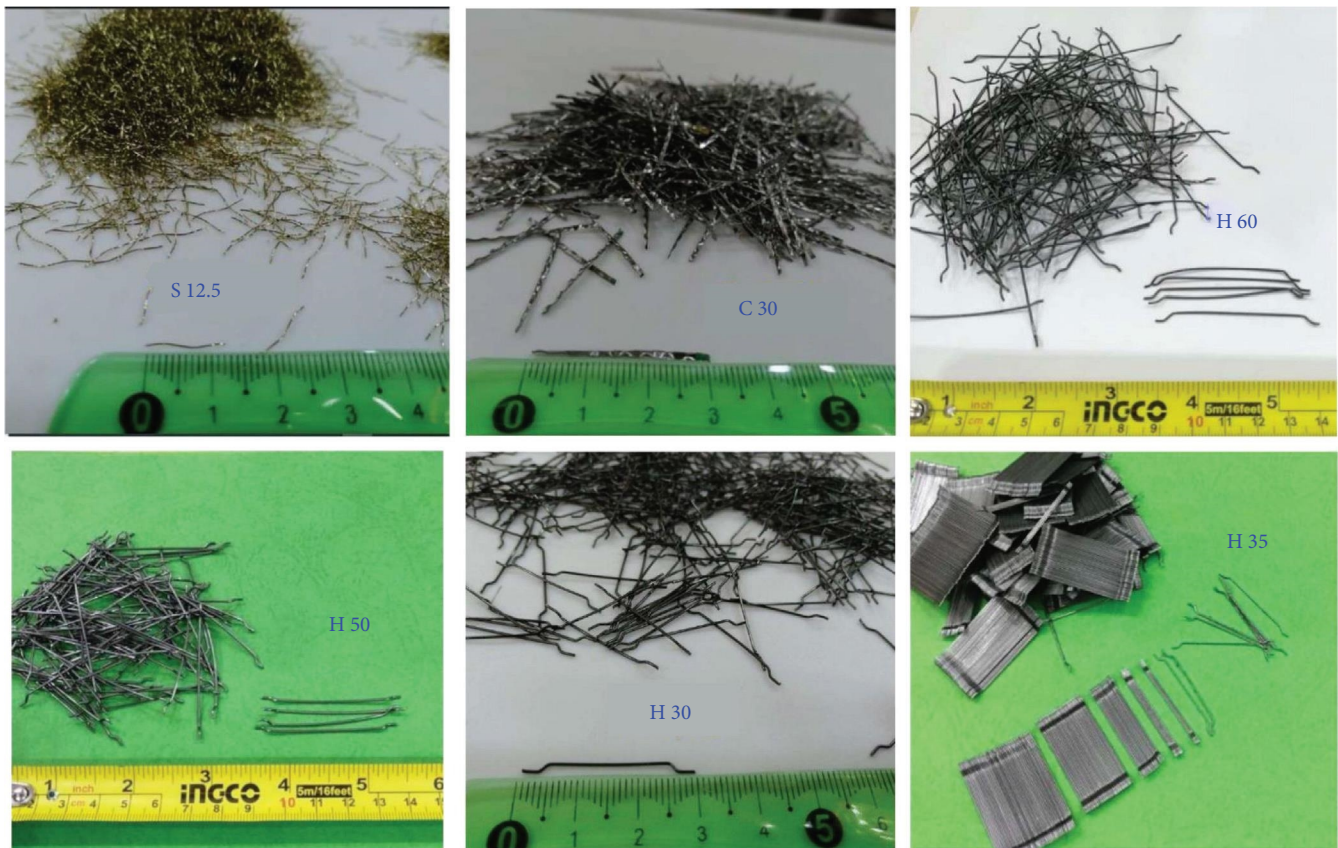
FIGURE 3: Represents the types of steel fibers.
