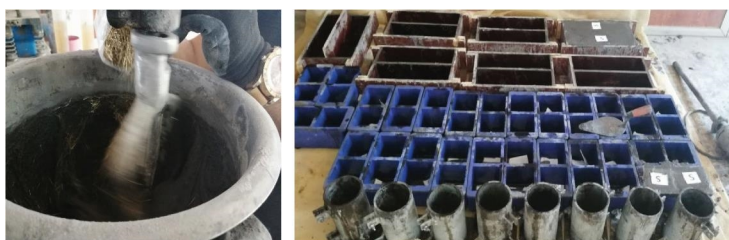
FIGURE 5: Mixing procedure and casting of RPC.
