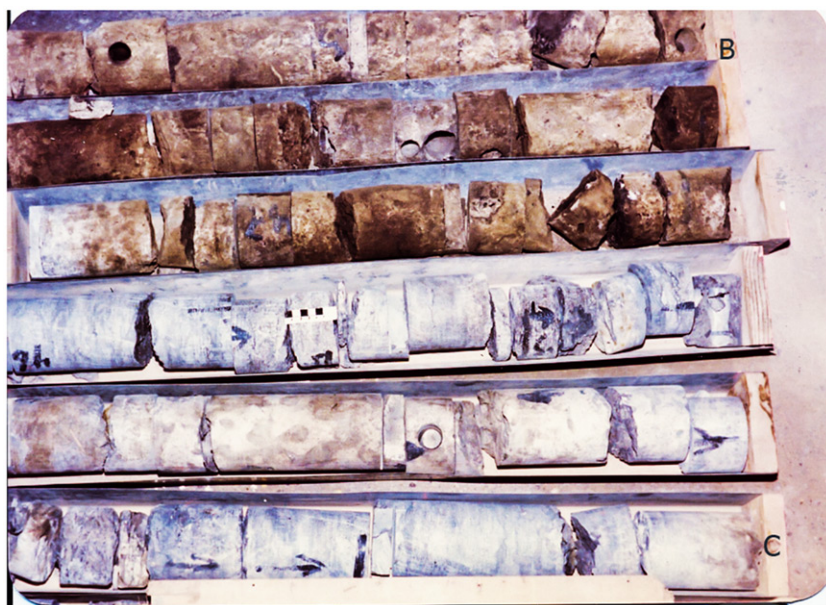
Figure 3. Cores from the Yamama Formation in the well West Qurna-15 showing an oil-stained reservoir unit at the top and argillaceous limestone barrier unit at the lower part. Core box length is 1 meter.
