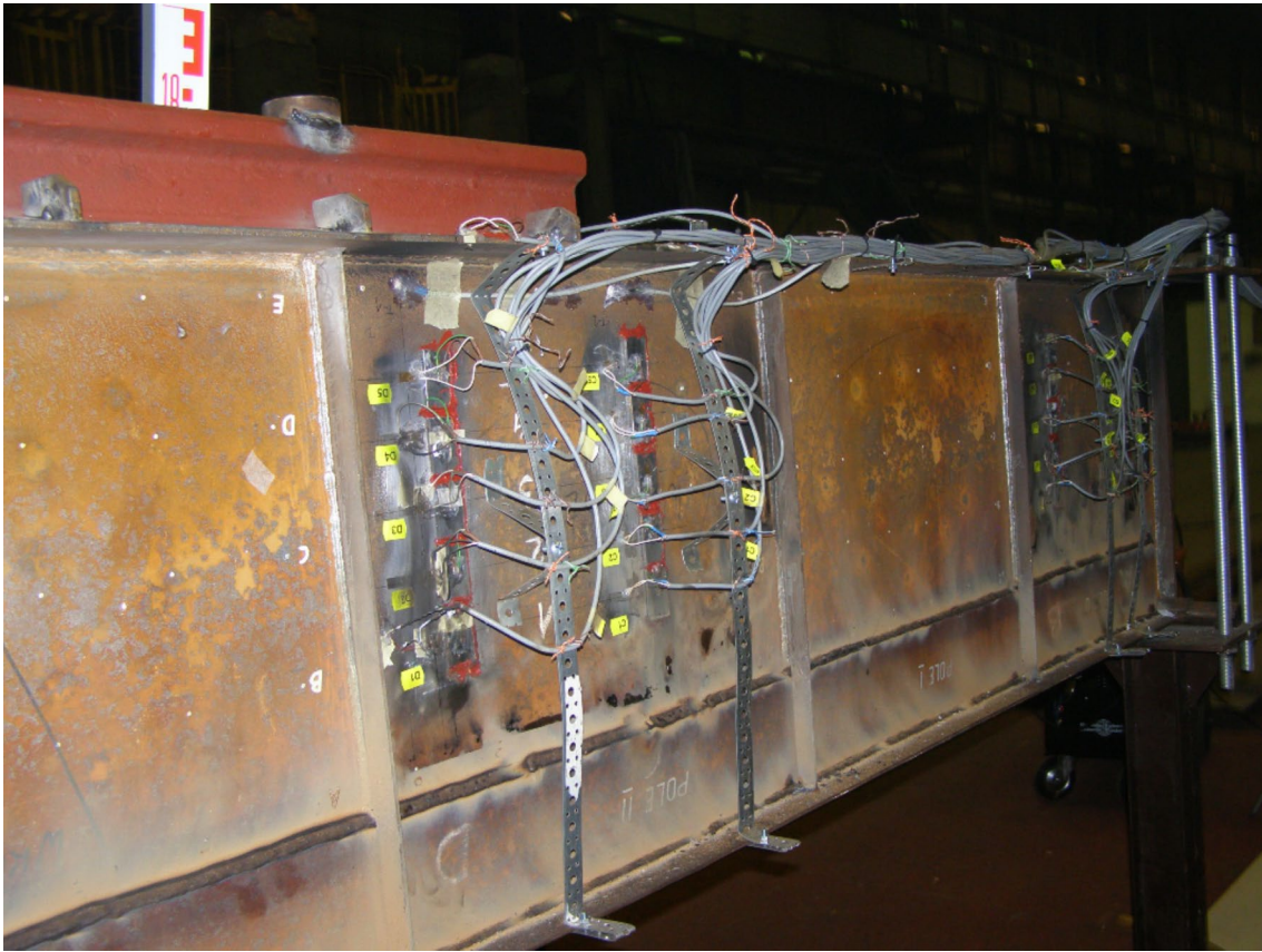
Fig. 4 Sensor's position on the girder after the technological prestressing process
