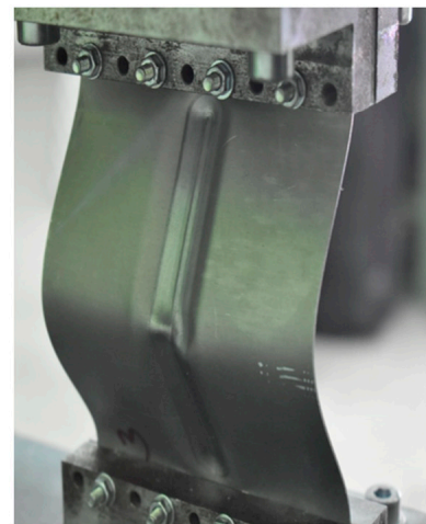
Figure 8. Aluminum alloy EN AW-2024-T3 sheets under compression load in different conditions.
