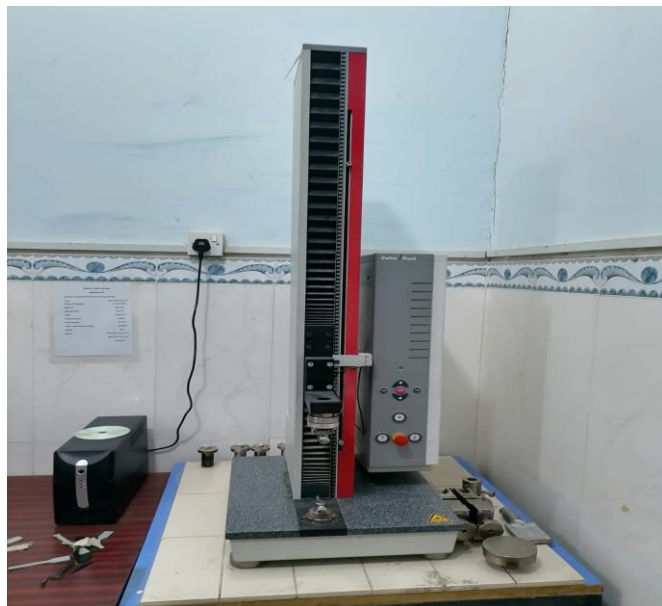
Figure 1. tensile strength test sample and mechanical properties measuring device (Tensile).
