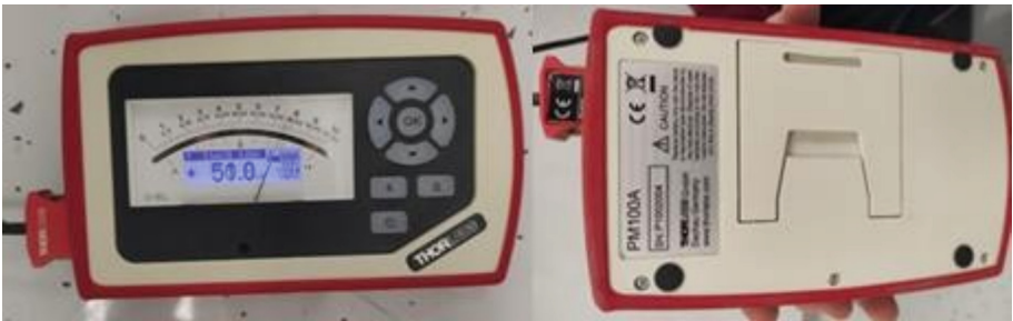
Fig. 6. Thorlabs PM10A optical power measurement instrument
