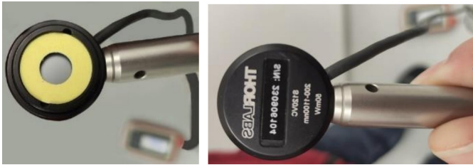
Fig. 5. Optical power detector Thorlabs PM100A (front and rear)
