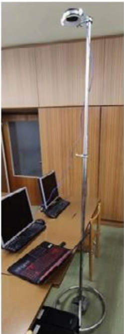
Fig. 9. Ensuring direct visibility between the USB Dongle and the LiFiMAX Photonic Antenna
