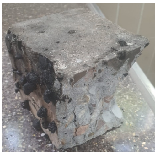
Fig. 21. Compressive strength test for SCCPVC10 after subjected to 300°C.
