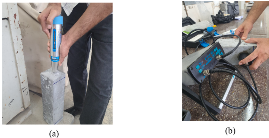
Fig. 6. Non-destructive tests: a) Schmidt rebound hammer, and b) ultrasonic pulse velocity (UPV).
