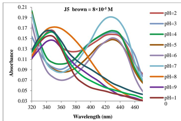
**Figure 4:** Absorption spectra at pH levels of 2-12.
