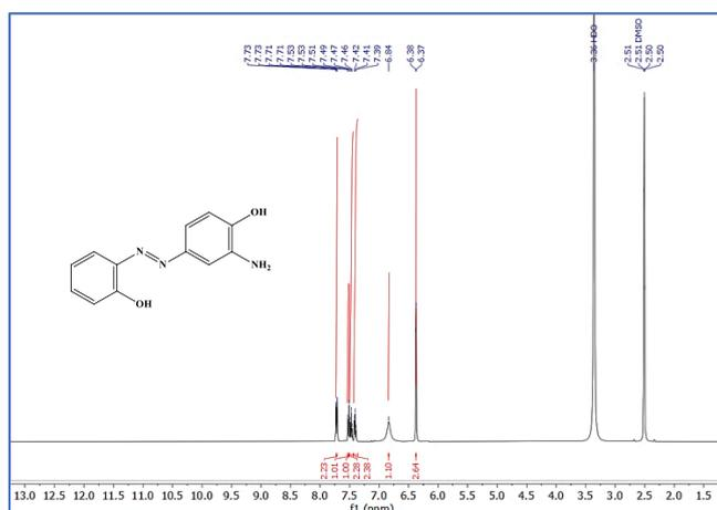
**Figure 2:** Proton nuclear magnetic resonance (<sup>1</sup>H NMR) spectra of the J5 brown dye.
