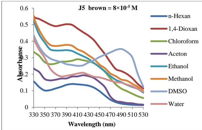
**Figure 6:** Electronic spectra of the J5 brown dye in different polar solvents.
