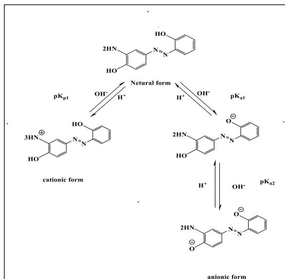
**Scheme 2:** Mechanism of the J5 brown dye.
