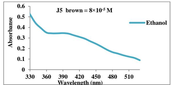
**Figure 8:** Spectral absorption for the J5 brown dye in ethanol.
