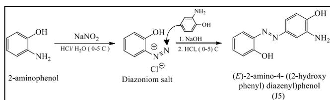
**Scheme 1:** Preparation of the azo J5 brown dye ((E)-2-amino-4-((2-hydroxyphenyl) diazenyl) phenol)
