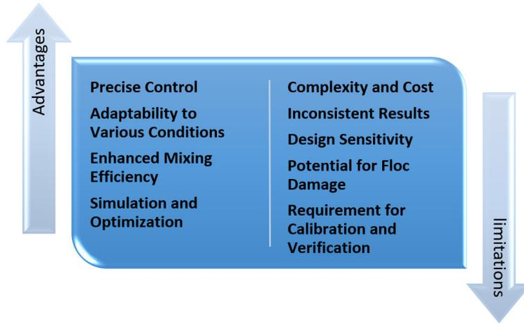
Figure 4. Advantages and Disadvantages of Mechanical Flocculators
