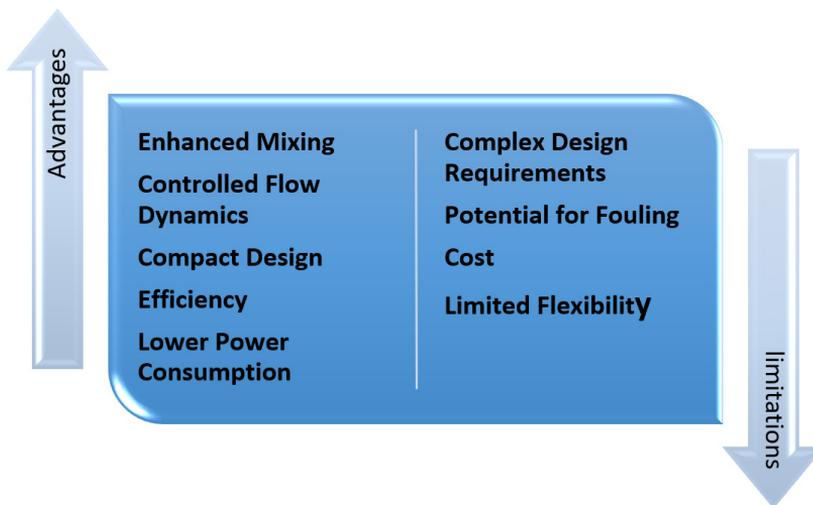
Figure 6. Advantages and Disadvantages of Helically Coiled Tube Flocculators
