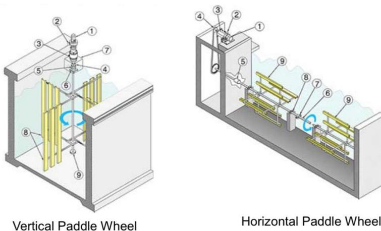
1-stirring column; 2-shafarah; 3-stirring rods; 4- rotary motor; 5- paddle-wheel flocculator; 6-comprises a turbine; 7-speed regulator; 8-three blades, driven direct
