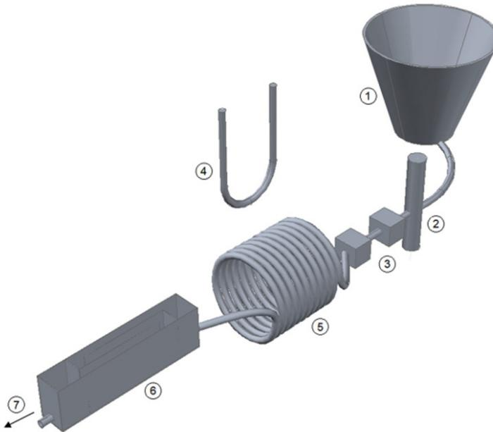
(1) a reservoir of synthetic water; (2) a flow meter (flow controllers); (3) dosing pumps of chemical reagents; (4) pressure gauge connected at flocculator's input and output sections; (5) flocculator; (6) decanter system (settling tank); and (7) drain to the final disposal of the fluid
