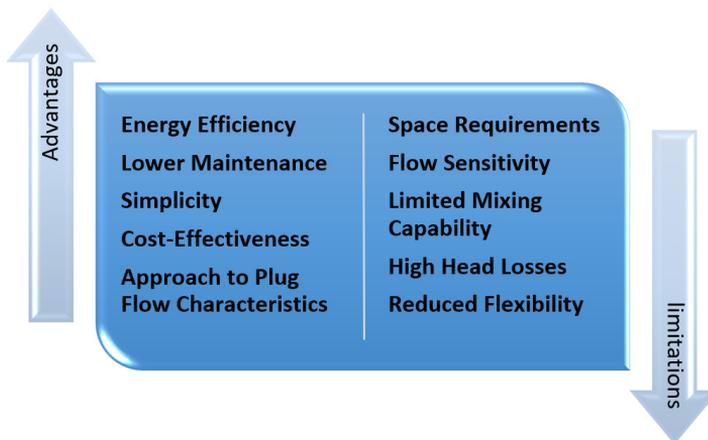
Figure 2. Advantages and Disadvantages of Hydraulic Flocculators
