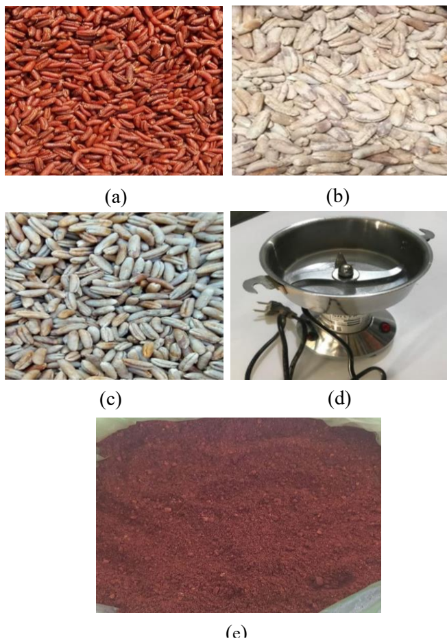
Figure 2. Date seed preparing process: a) washing and cleaning the date seed, b) after drying under the sunlight, c) after drying in the oven, d) the grinder used for finning the size, e) final result
