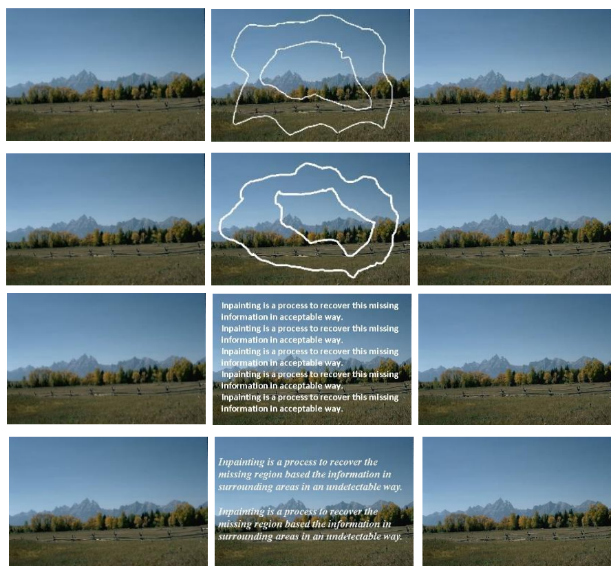
Figure 3: Inpainting based transport equation in spatial domain, column 1 original images, column 2 masked images, column 3 inpainted images.
