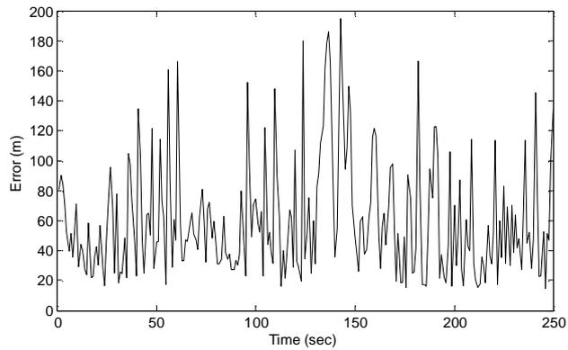
Fig.6b: The rms error of the two stage Kalman filter of scenario2.
