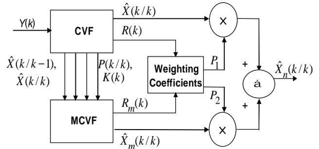
Fig. 1: The proposed tracking system for one coordinates (range).
