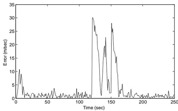
Fig.4a: The rms range rate error of the CVF of scenario1.
