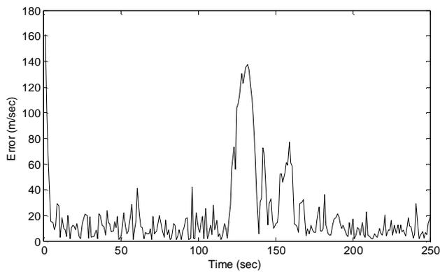
Fig.4b: The rms range rate error of two stage Kalman filter of scenario1.
