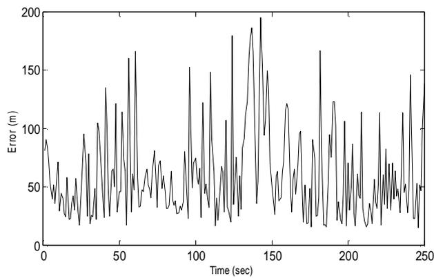
Fig.3b: The rms error of the two stage Kalman filter of scenario 1 .
