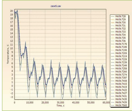
Fig. 10. Magnetorquer Temperature Profile Note the cyclical heating and cooling experienced by the Magnetorquer. It takes approximately four orbits for the Magnetorquer's average temperature to stabilize and it shows that minimum temperature at -4\text{ }^{\circ}\text{C}
