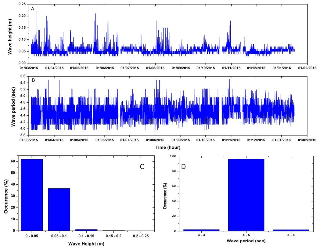
Figure 5. Hourly wave height (A), hourly wave period (B), percentage of various wave height classes (C) and percentage of various wave period classes (D)
