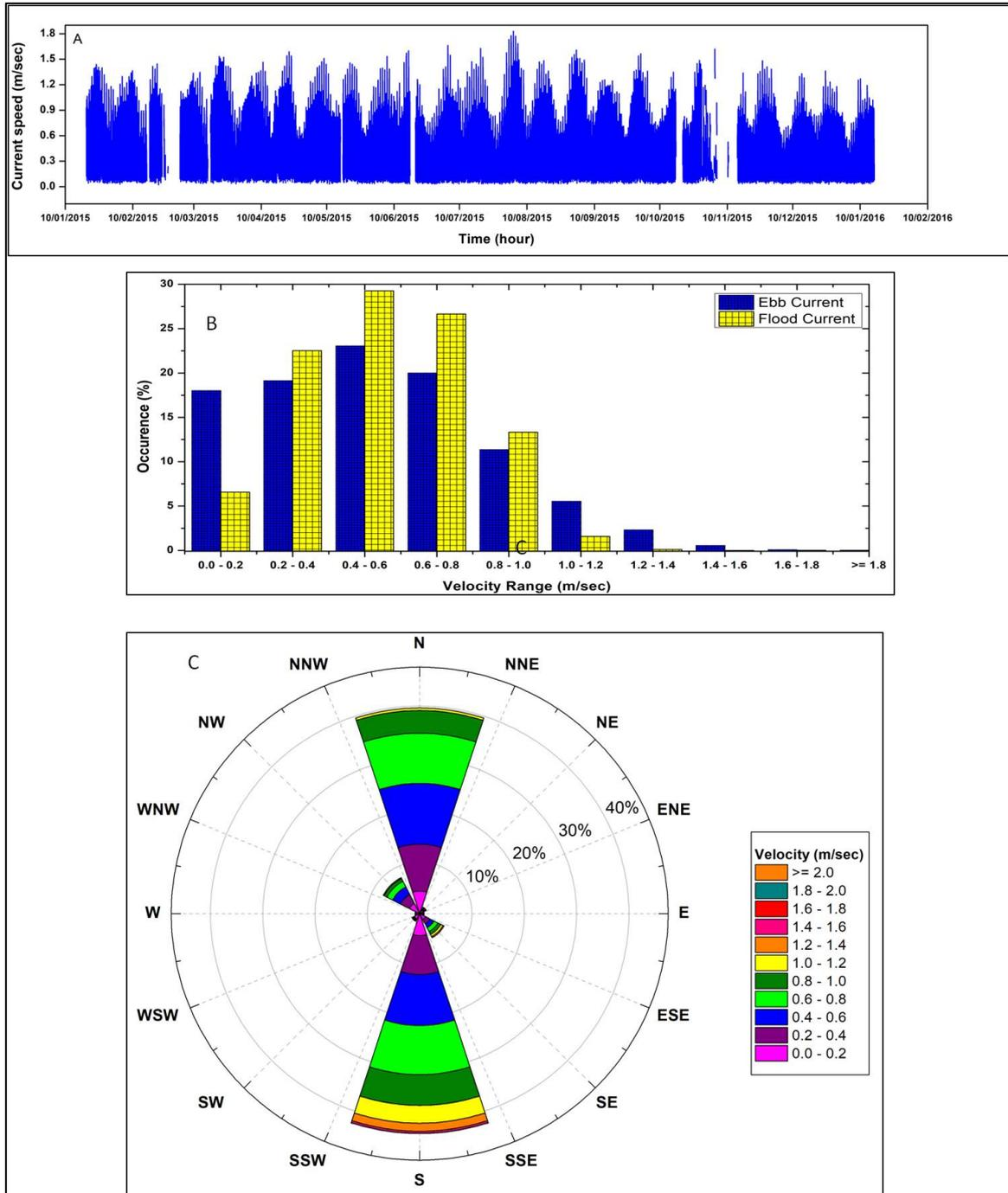
Figure 3. Current speed (A), frequency of various velocity classes for flood and ebb current (B), current rose (C)
