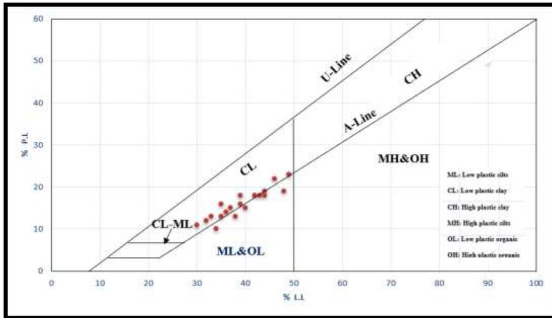
**Fig. 3. Plasticity as per the USCS classification scheme for study area soils (ASTM D 2487-17).**
