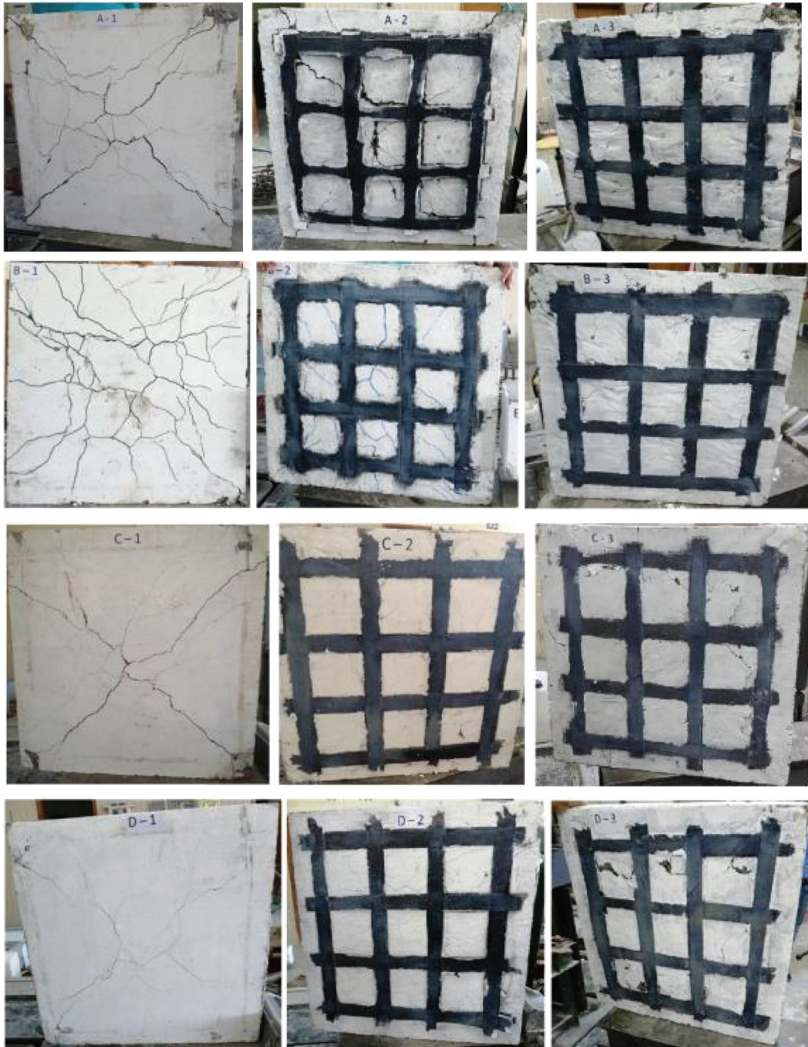
FIGURE 10: Cracks' patterns and mode of failure.
