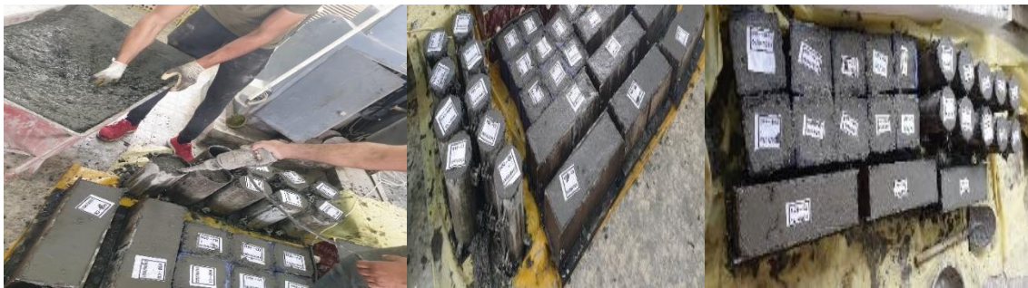
Fig (3-7) Casting, levelling, labelling of the standard steel molds.
