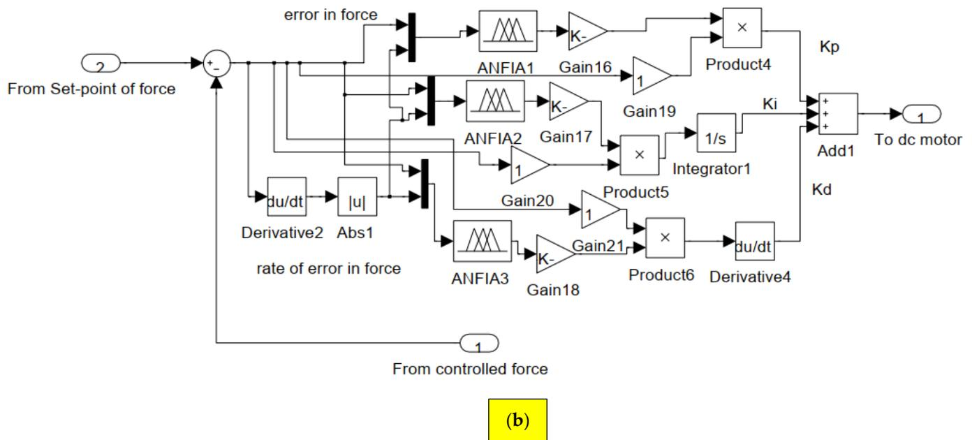
**Figure 7.** Simulink model of ANFIS-PID controller: (a) in developing the gripper position control and (b) in developing the gripper force control.
