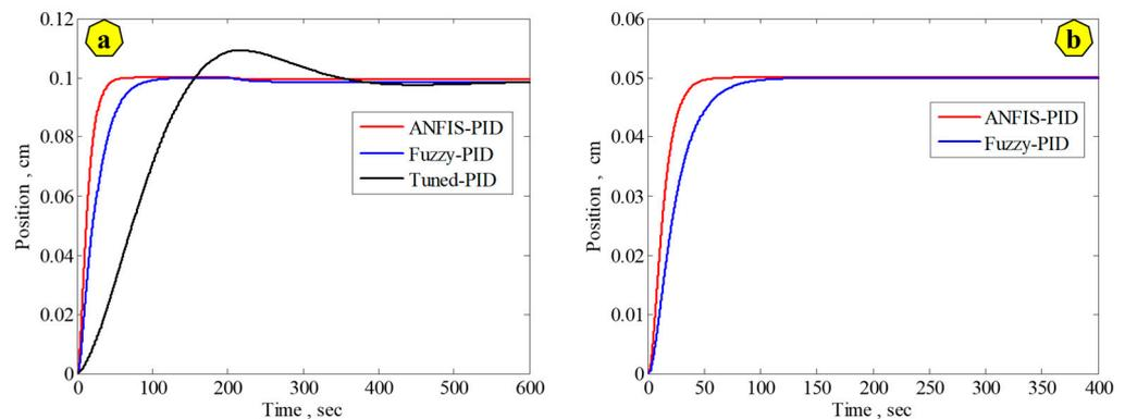
**Figure 19.** (a) Effect of disturbance on the ANFIS-PID, Fuzzy-PID, and Tuned-PID controllers, (b) precision movement of gripper during ANFIS-PID and Fuzzy-PID controllers.
