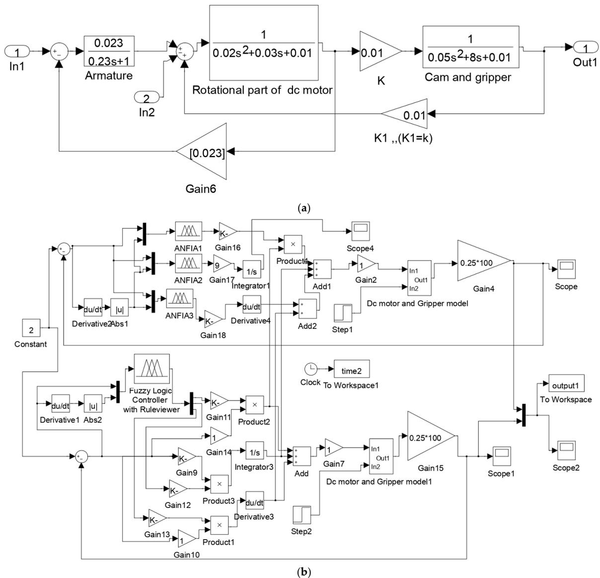
Figure 17. (a) The Simulink model of the system (motor, cam, and gripper). (b) Applying the proposed ANFIS for gripper position control.
