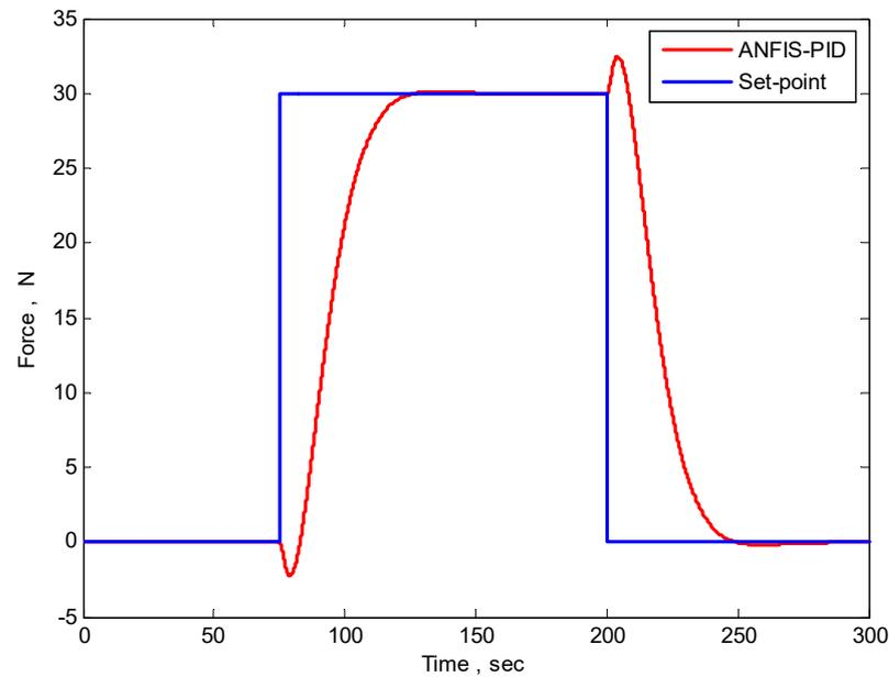
**Figure 28.** Force control by the proposed ANFIS-PID when the set point drops from 30 N to 0.
