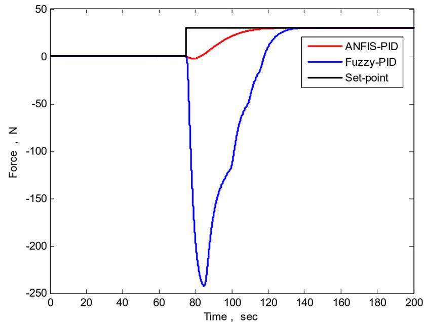
**Figure 25.** The performance comparison between the proposed ANFIS-PID and the Fuzzy-PID in controlling a required force of 30 N (set point).
