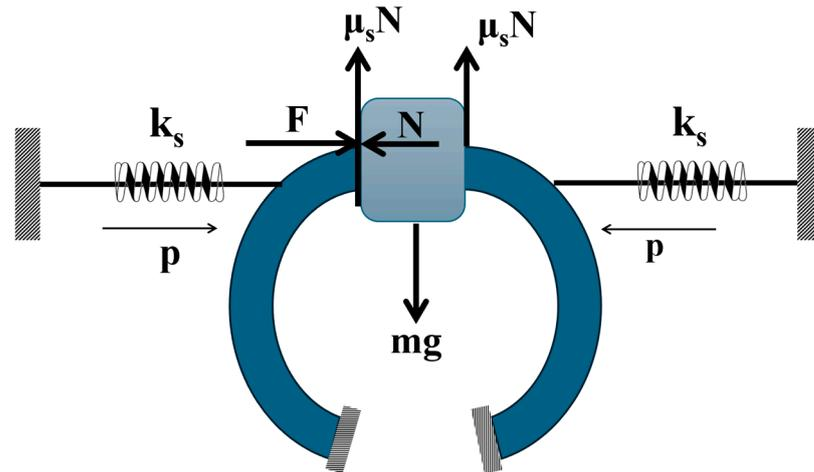
**Figure 22.** A mathematical model of force representation on the proposed gripper.
