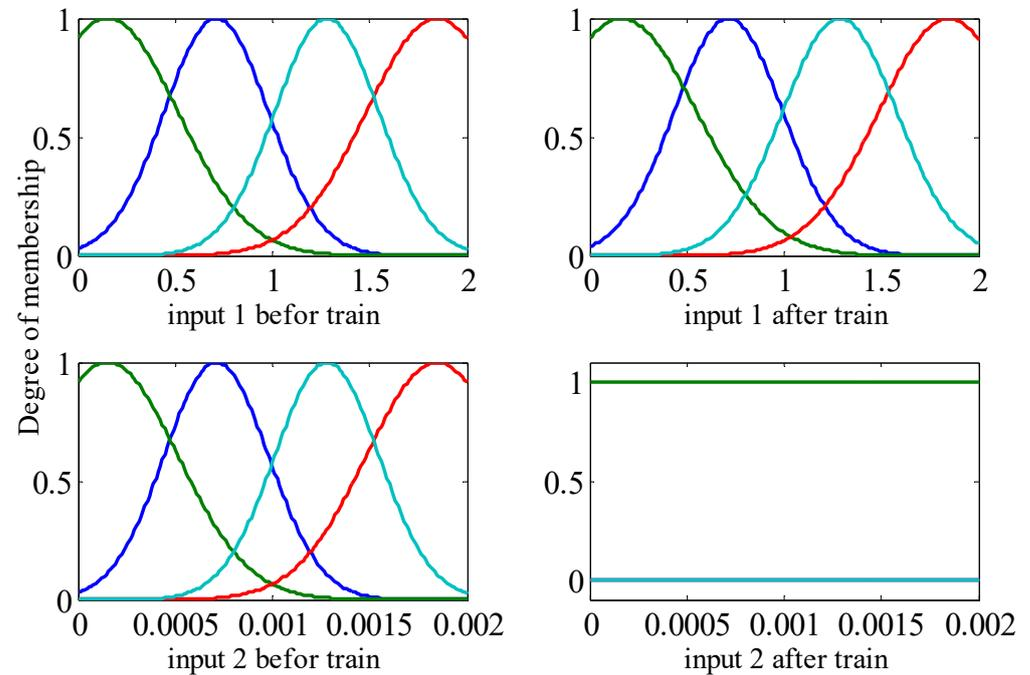
**Figure 14.** Input membership functions before and after training using *genfis3*. The unit of measuring input 1 (position error) is cm; that for input 2 (derivative of error) is cm/s. The degree of membership is dimensionless.
