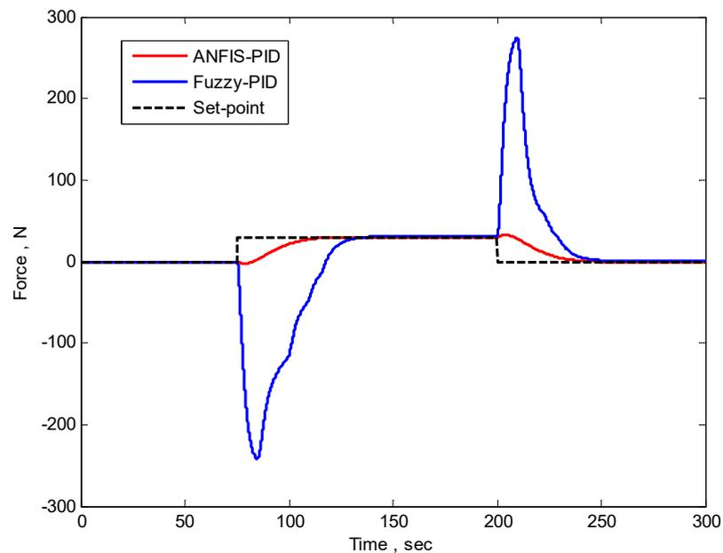
**Figure 29.** The comparison between the proposed ANFIS-PID and the Fuzzy-PID when the set point drops from 30 N to 0.
