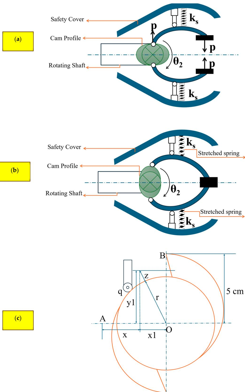
**Figure 4.** The main construction of the system. (a) The open case of the proposed gripper, (b) the closed case of the proposed gripper, and (c) the cam profile.
