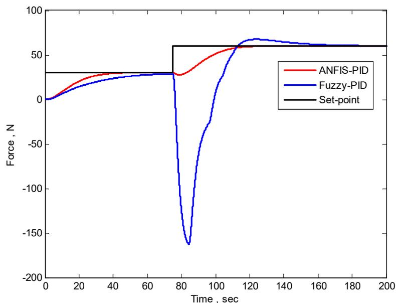
**Figure 27.** The performance comparison of the proposed ANFIS-PID and the Fuzzy-PID using two set points of forces or when there is a change in the required force from 30 to 60 N.
