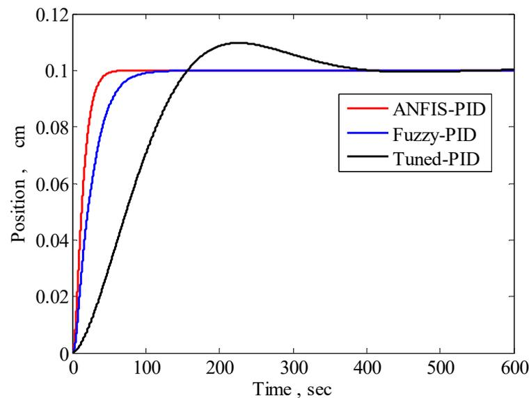
**Figure 18.** Position variation comparison between ANFIS-PID, Fuzzy-PID, and Tuned-PID controllers.
