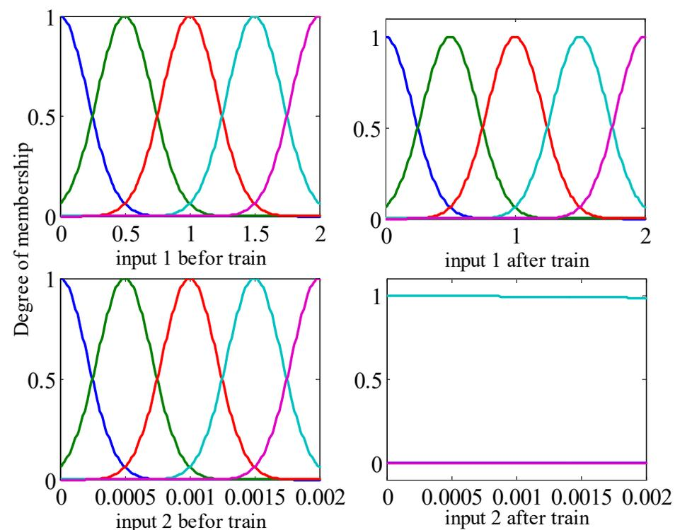
**Figure 8.** Inputs of membership functions before and after training using *genfis1*. The unit of measuring input 1 (position error) is cm; that for input 2 (derivative of error) is cm/s. The degree of membership is dimensionless.
