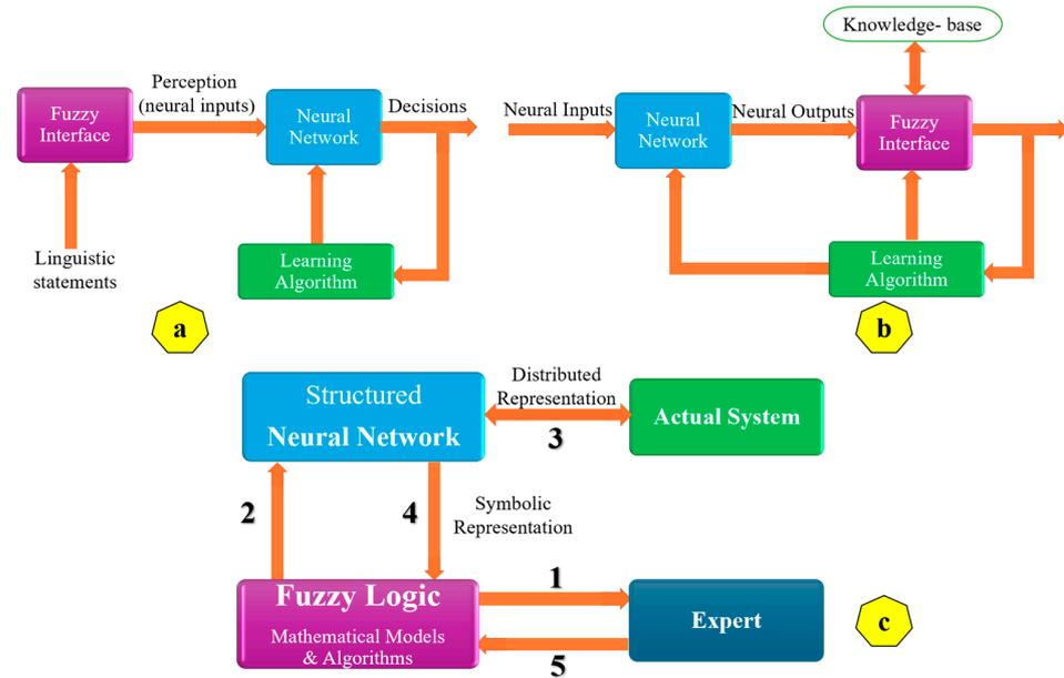
**Figure 2.** Structures of several fuzzy neural systems. (a) The fuzzy interface block acts as an input to a neural network, (b) A neural network drives the fuzzy inference mechanism, and (c) Neural network's function in neuro-fuzzy techniques to tune membership functions in system.
