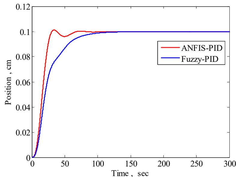
**Figure 21.** Precision movement of the gripper in the developed ANFIS-PID and Fuzzy-PID controllers.
