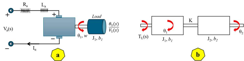
**Figure 5.** Schematic of the (a) DC motor loading and (b) torque effect on the DC motor.  $w$  represents the angular speed of the motor.
