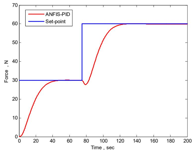
**Figure 26.** The performance of the proposed ANFIS-PID control using two set points of forces or, in other words, when there is change in the required force from 30 N to 60 N.
