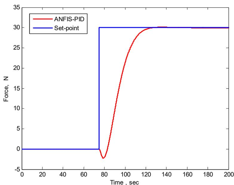
**Figure 24.** Force control by the proposed ANFIS-PID to achieve a required force (set point) of 30 N.
