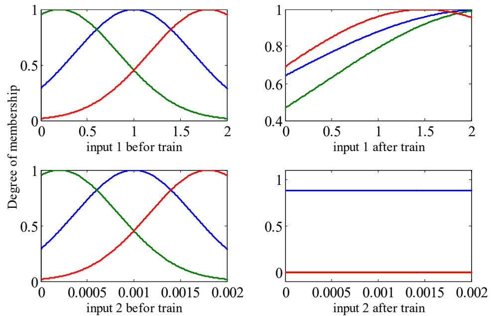
**Figure 11.** Input membership functions before and after training using *genfis2*. The unit of measurement for input 1 (position error) is cm; that for input 2 (derivative of error) is cm/s. The degree of membership is dimensionless.
