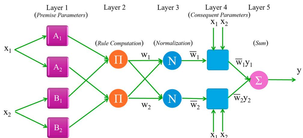
**Figure 3.** Adaptive network-based fuzzy inference system (ANFIS).
