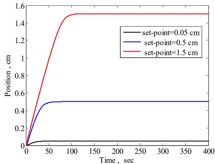
**Figure 20.** Testing of developed ANFIS-PID controller at different set points.
