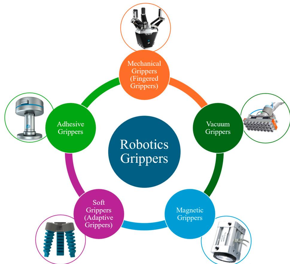
**Figure 1.** Main robotic grippers classified by working principle.
