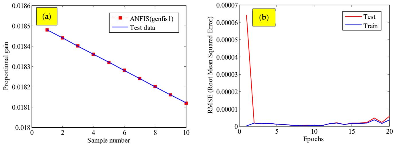
Figure 10. ANFIS *genfis1*: (a) prediction test, (b) root-mean-squared error (training and testing).
