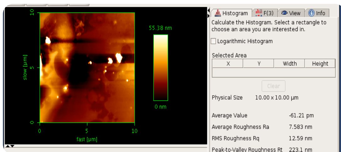
Figure showing AFM analysis of zinc oxide nanoparticles manufactured from naringenin nanoparticles
