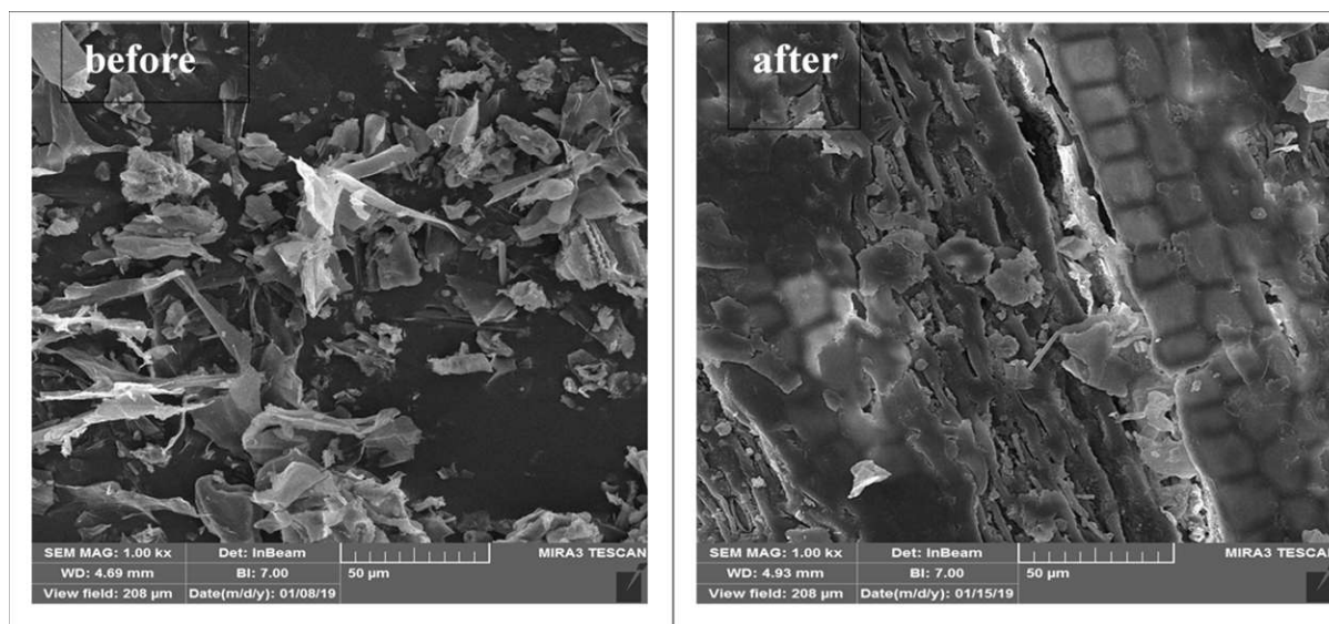
(Picture 1) SEM for the Typha biomass before and after lead adsorption
