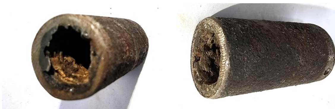
Figure 15. Sample of defective heat exchanger pipe before treatment
