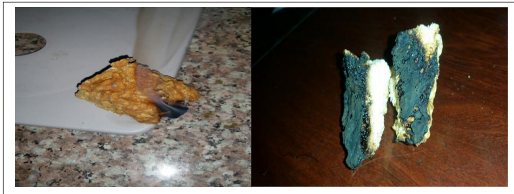
Figure 2: The combustion test of fabricated panels core.
