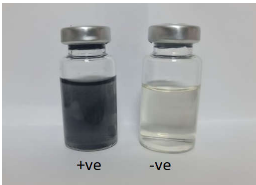
(Figure 1) Black precipitates of iron sulfide
