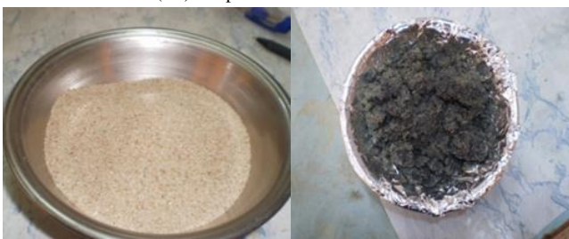
Fig. 10. Visual comparison of clean sand (left) and bio-particles (right)
