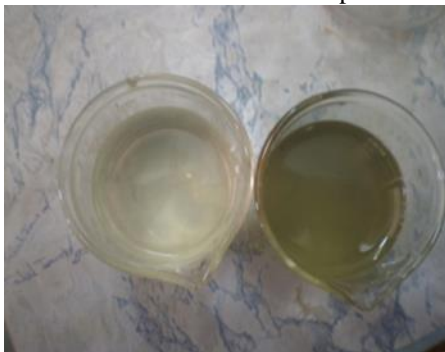
Fig. 9. Visual comparison of influent (right) and effluent (left) samples
