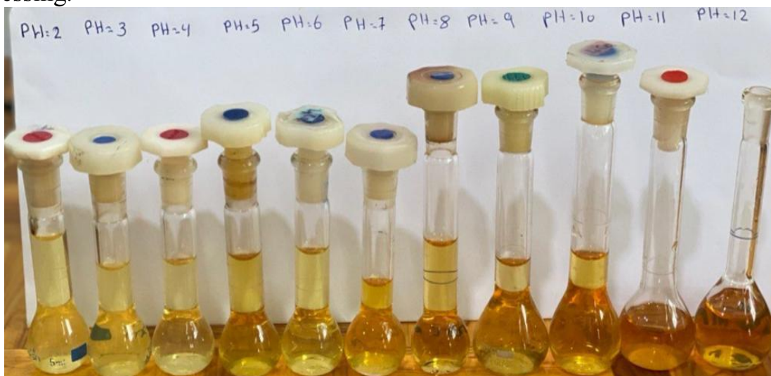
Fig 9. Color change of solution of azodyes A at various buffer solution with pH 2–12
