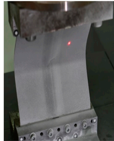
(b) Applying 8kN on 3mm thickness
