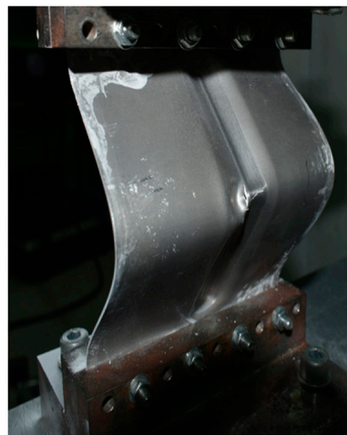
Figure 8. Aluminum alloy EN AW-2024-T3 sheets under compression load in different conditions.
