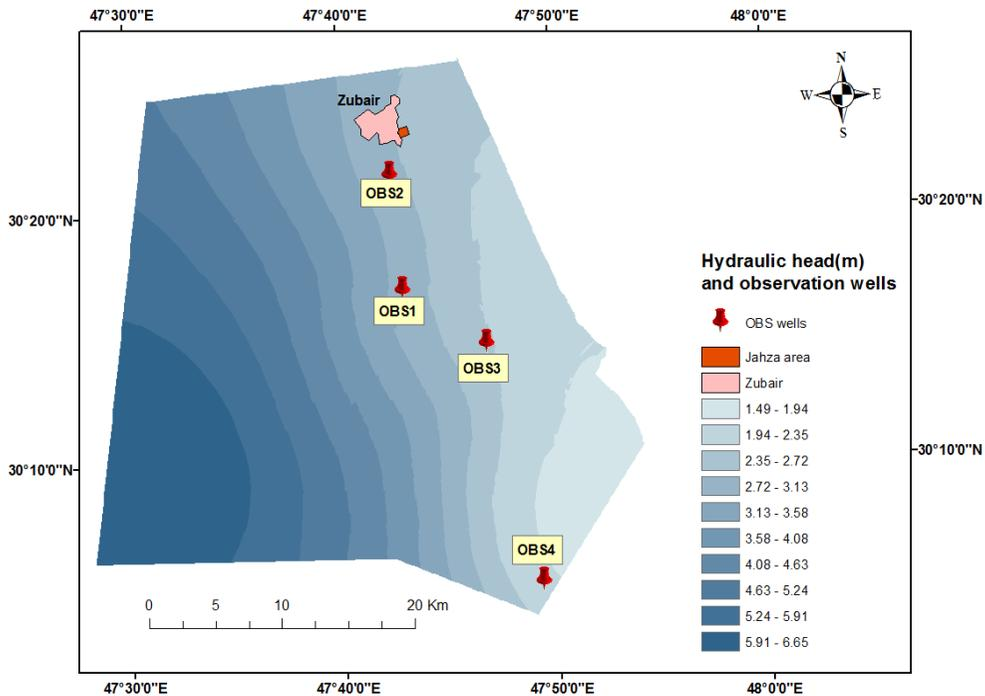
Figure 5. Initial hydraulic head and observation wells.
