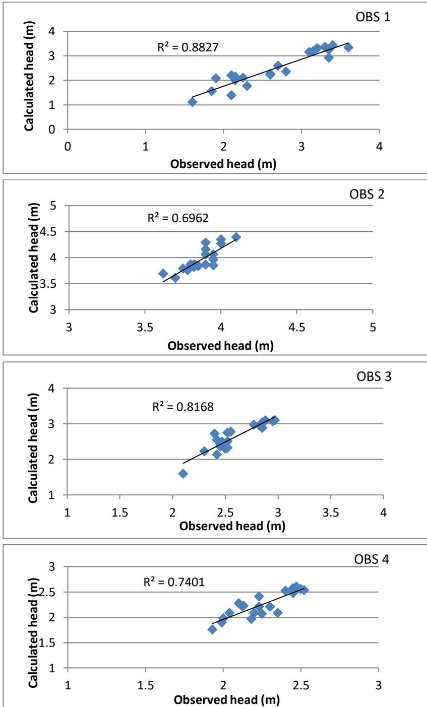
Figure 7. The determination coefficient ( $R^2$ ) between the observed and calculated heads.
