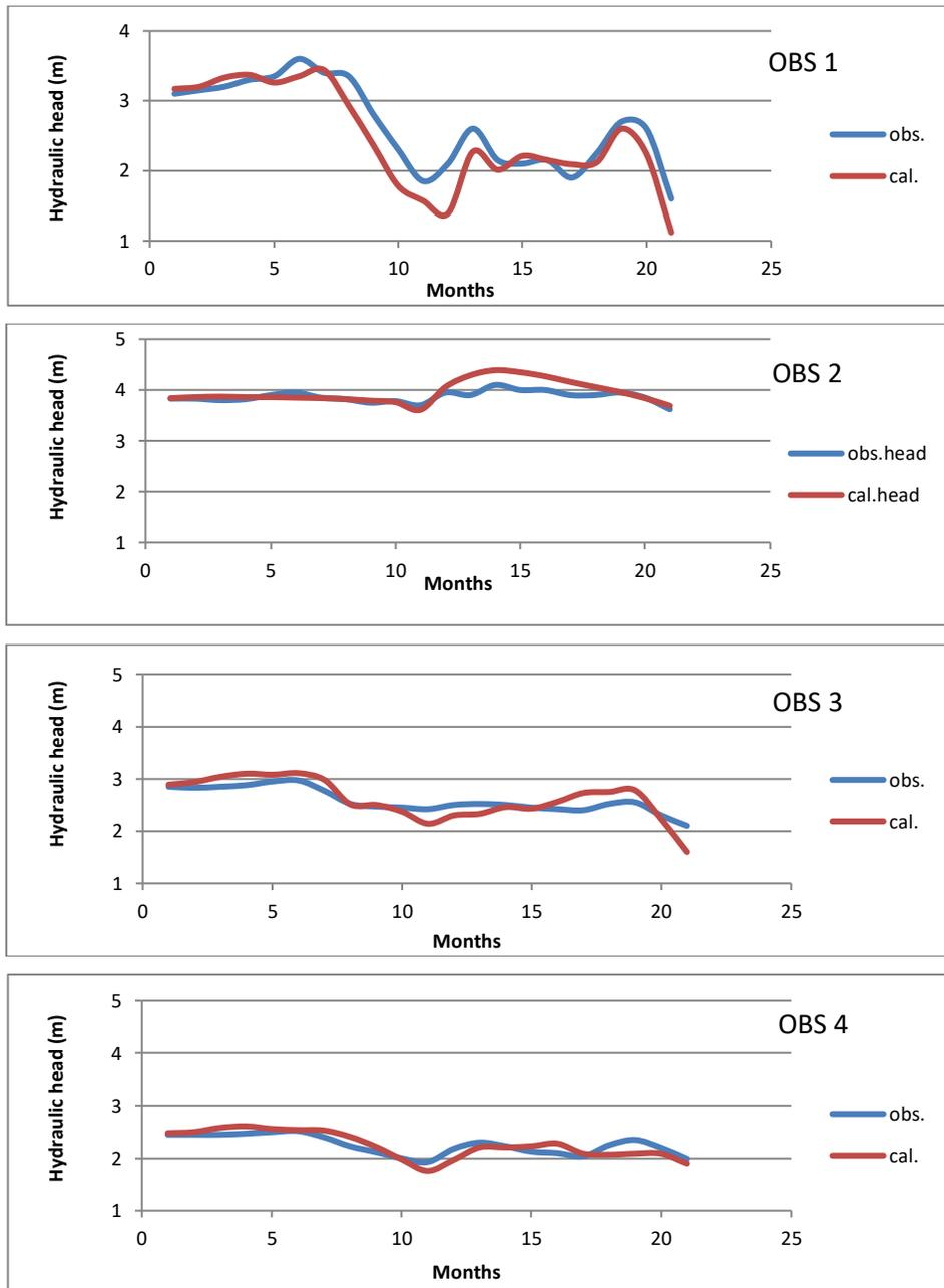
Figure 6. A comparison between the observed and calculated heads.
