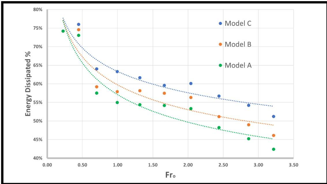
FIGURE 6. Relationship between energy dissipated and  $Fr_o$
