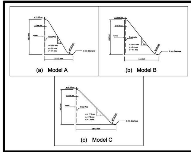
FIGURE 1. Sketches of experimental ogee models
