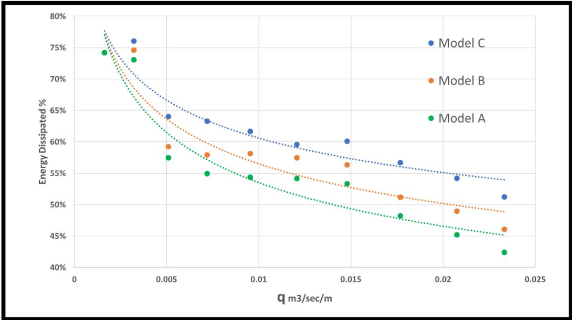
FIGURE 5. Relationship between energy dissipated and discharge per unit width
