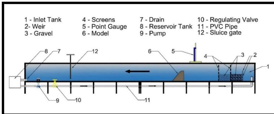
FIGURE 2. Detailed drawing of a laboratory flume
