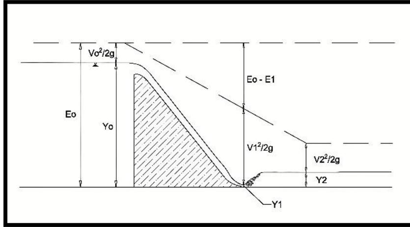
FIGURE 4. Details of energy lines
