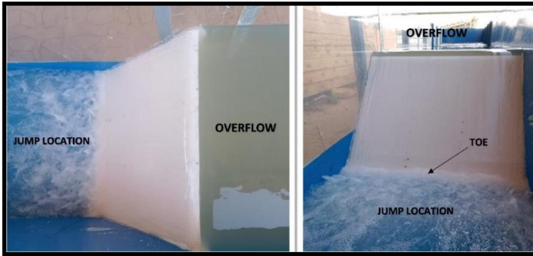
FIGURE 3. Flow over ogee spillway and jump location
