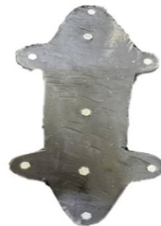
Fig.5. The Teflon rubber piece that is placed under the base of the shoe.
