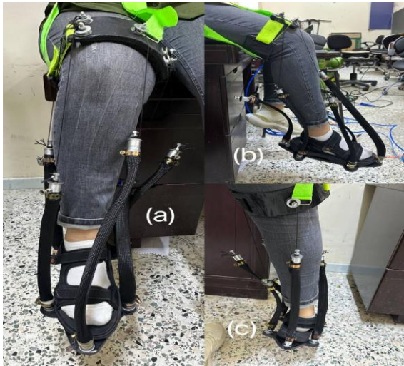
Fig.11. The integrated shape of the robot. (a)The shape of the robot and the frontal muscle. (b) The shape of the robot from the side and the lateral muscles. (c) The shape of the robot and the back muscle
