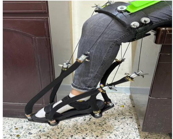
Fig.9. The six muscles are attached to the threads from the top with pieces of Teflon around the thigh from the top.
