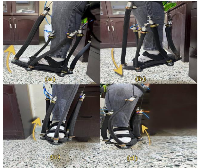
Fig.12. The robotic movements of the ankle joint (a) Forward motion of the ankle. (b) Posterior movement of the ankle. (c) Movement towards the right of the ankle. (d) Movement towards the left of the ankle joint
