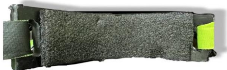
Fig.8. A piece of light and soft sponge is placed inside the piece around the thigh.
