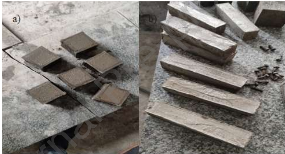
Figure. 3 (a) CQDs-cement Mortar cubes for the compression test, (b) CQDs-cement mortar prisms for the flexural test.
