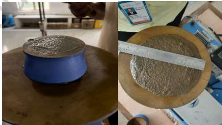
Figure. 2 Mini-Conical Slump Flow Test
