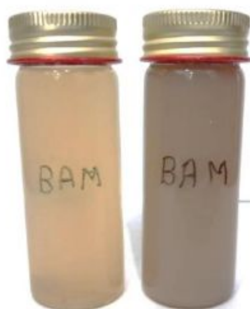
Fig. (2): The change in colour of the reaction solution indicates the manufacturing of silver nanoparticles using A. esculentus fruit aqueous extract.
