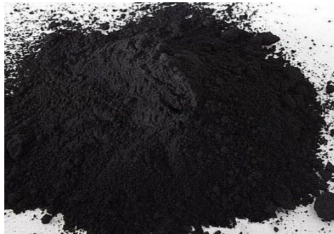
Figure 2: Vulcanized rubber (car tire rubber powder waste).
