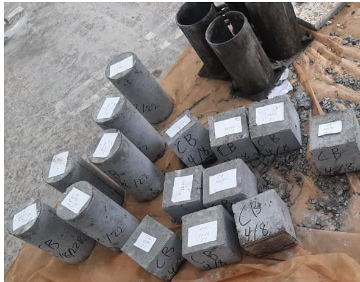
c. Cylinder and cubes extracted from their molds.
