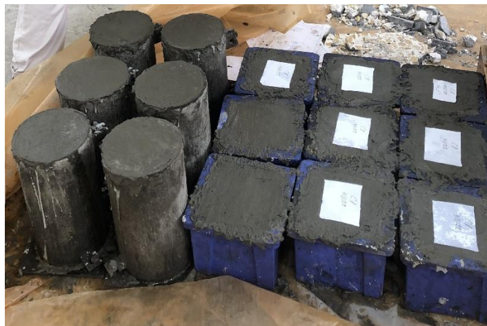
b. leveling and marking the cubes and cylinders.
