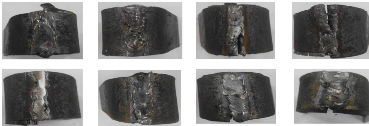
FIGURE 11. Bending test for samples without any crack for welding condition of case study number 1-1, 1-3, 2-2 and 3-5
