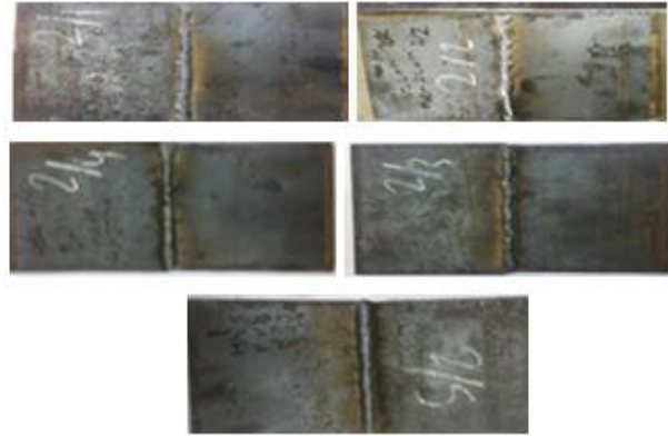
FIGURE 3. Carbon steel plate welded with 18 V, 10 l/min CO 2 , wire welding speed from 8.5 m/min and different current from 10 to 100 Amp
