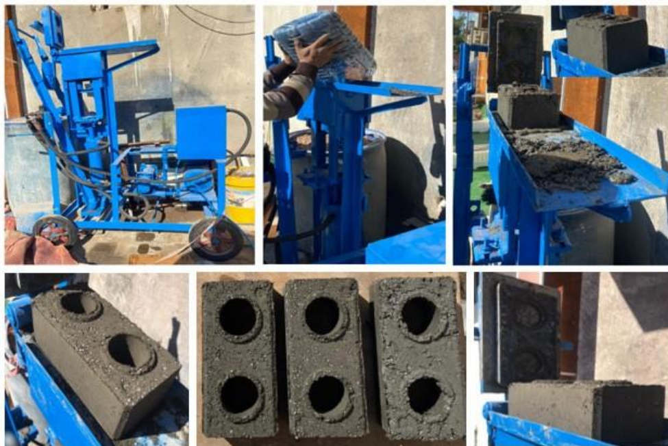
Figure 3. Pressing of polyethylene or polypropylene waste with cement mixture
