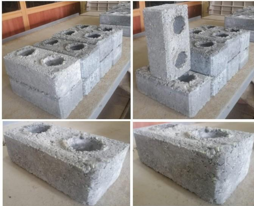
Figure 5. Plastic reinforced bricks Samples produced by using plastic waste
