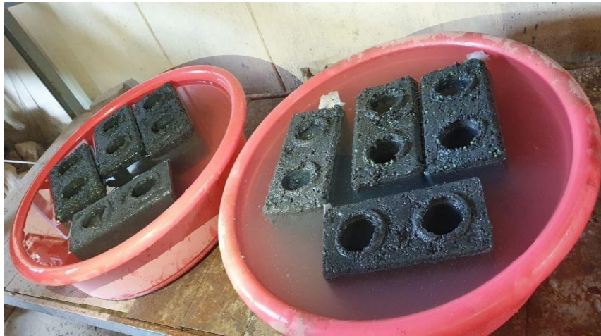
Figure 4. Plastic blocks in water dipping
