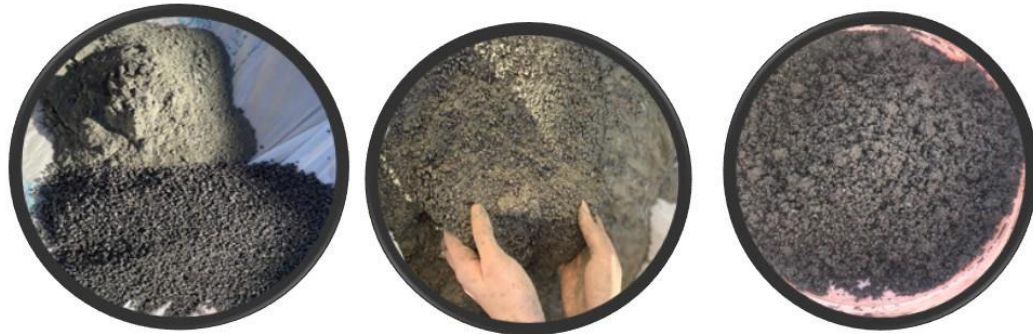
Figure 2. Prepare and mix polyethylene or polypropylene waste pellets with Portland cement
